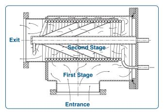
Figure 1 — Patented Vapor Sublimation Trap Design
