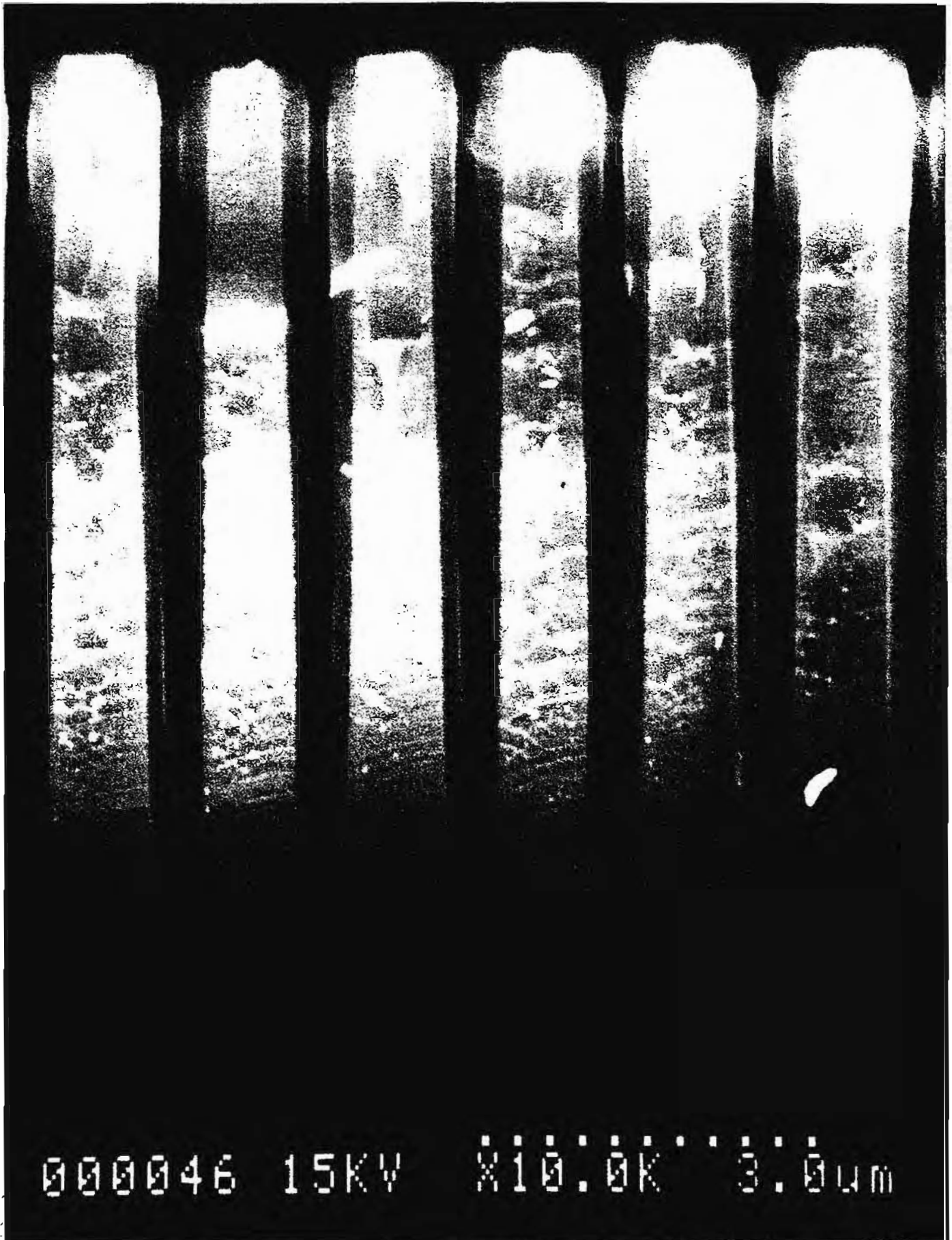
Fig. 9. 30 Torr, F-teos=80 sccm, F-O3=160 sccm, F-O2=3000 sccm, F-N2=1000 sccm, T=490 C
