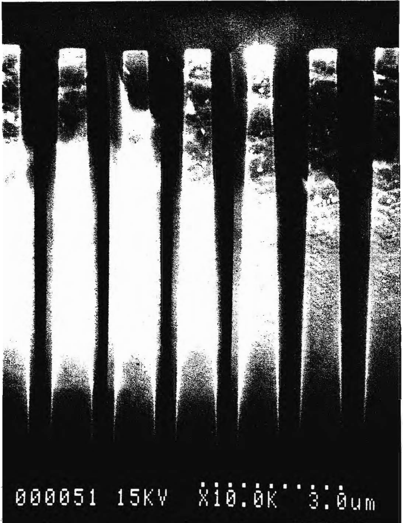
Fig. 7. 30 Torr, F-teos=80 sccm, F-O3=160 sccm, F-O2=3000 sccm, F-N2=10.0 sccm, T=415 C
