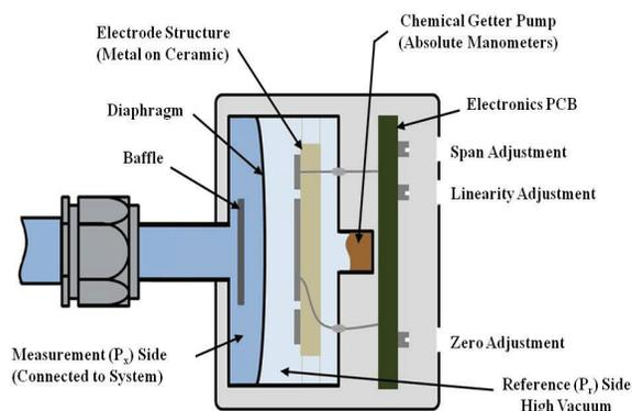
Figure 1 - Capacitance manometer schematic showing the internal components and functional zones
