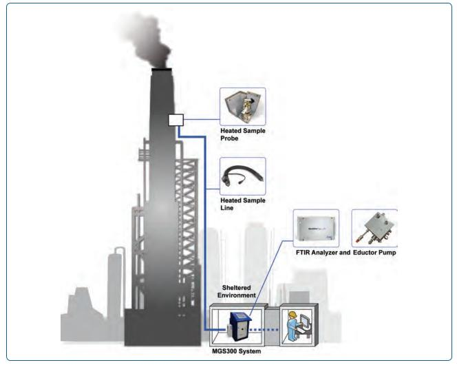
**CEMS Kit Component Diagram** — Illustrating layout and location of integrator kit modules
