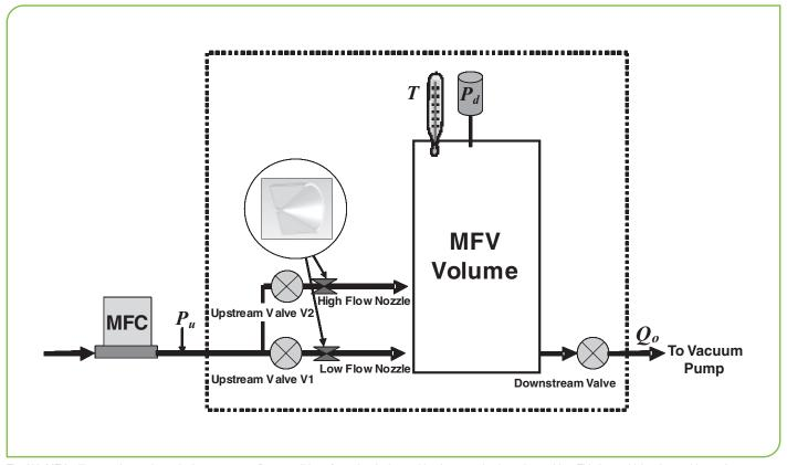
The HA-MFV utilizes sonic nozzles to isolate upstream flow conditions from the device making it external volume insensitive. This insensitivity along with precise temperature, pressure and volume measurements enables the device to provide measurement accuracies of better than 1.0% of Reading.
