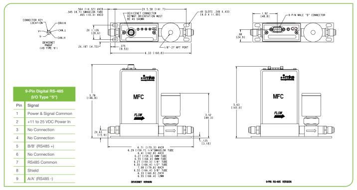
DeviceNet<sup>31</sup> and RS485 with VCR fittings\* (\*see manual for additional I/O and fitting types). Unless otherwise specified, dimensions are nominal values in inches (mm referenced).
