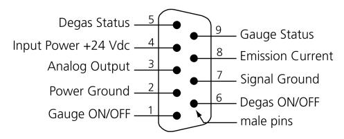
Figure 4-1: 9-pin Connector Pin Assignments
