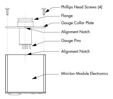
Figure 6-4 Mini-Ion Gauge Removal.
