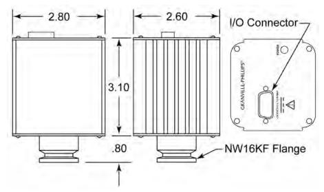
Figure 3-1: Series 342 & 343 Mini-lon Gauge Dimensions
