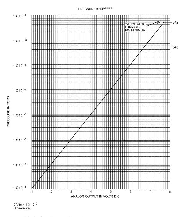
Figure 5-2: Analog Output in Volts dc
