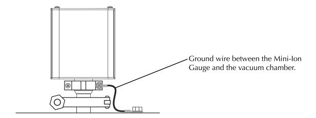
Figure 4-2: Grounding the Mini-lon Gauge to the Vacuum Chamber
