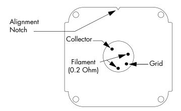
Figure 6-2 Mini-Ion Gauge Pin Identification.
