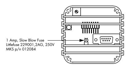
Figure 6-3 Position of 1 Amp, Slow Blow Fuse.
