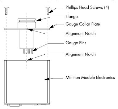
Figure 6-1 Mini-lon Gauge Removal.
