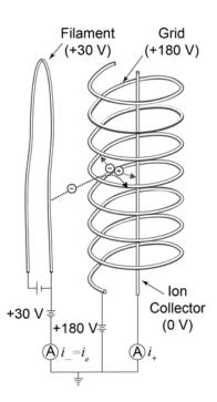
Figure 5-1: Typical Ion Gauge Schematic
