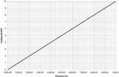
Analog out calibration = 11 (MKS Baratr The 1 Torr Baratron emulation provides a s \_ 10 VDC at 1 Torr.
