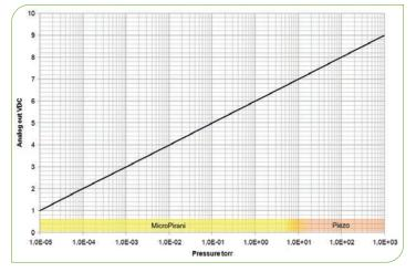
Standard Analog Output Pressure vs Voltage
