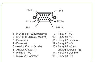
Pinouts Three (3) set point relays and dual Aout
