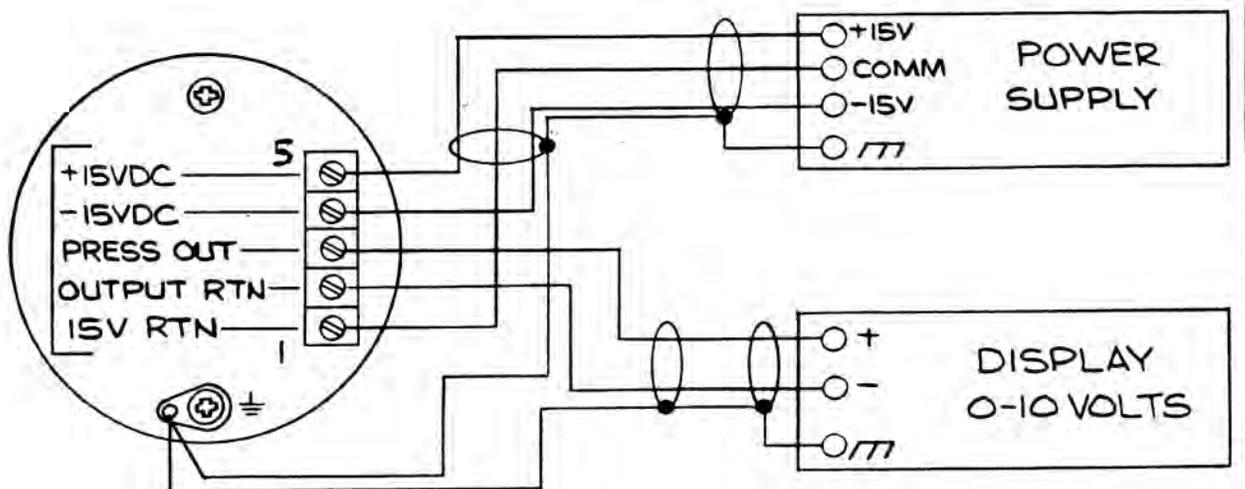
Figure 2: Electrical Connections
