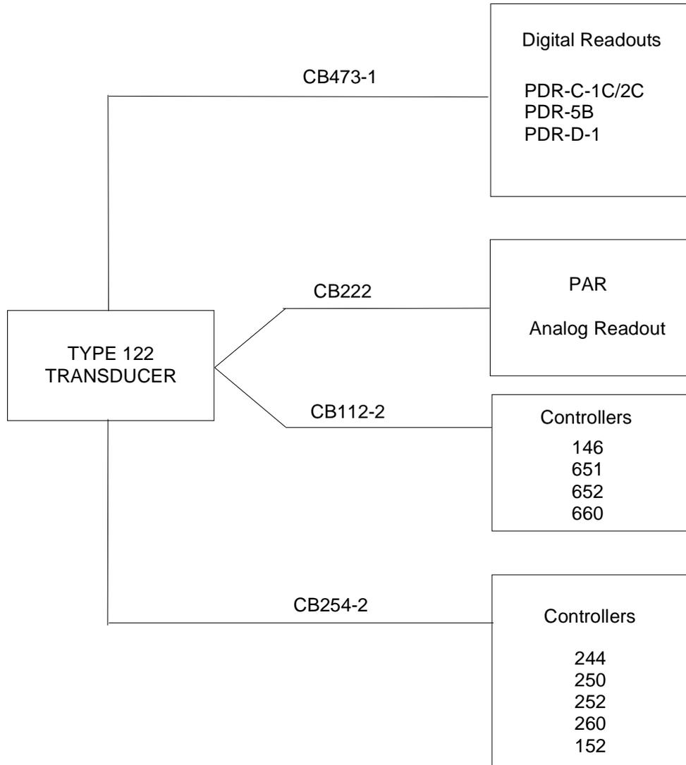
Figure 3: Interface Cables for the 122 Transducer
