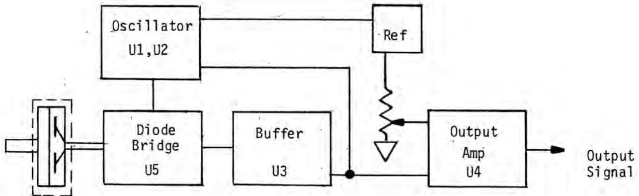
Figure 6: Block Diagram of the 122 Transducer
