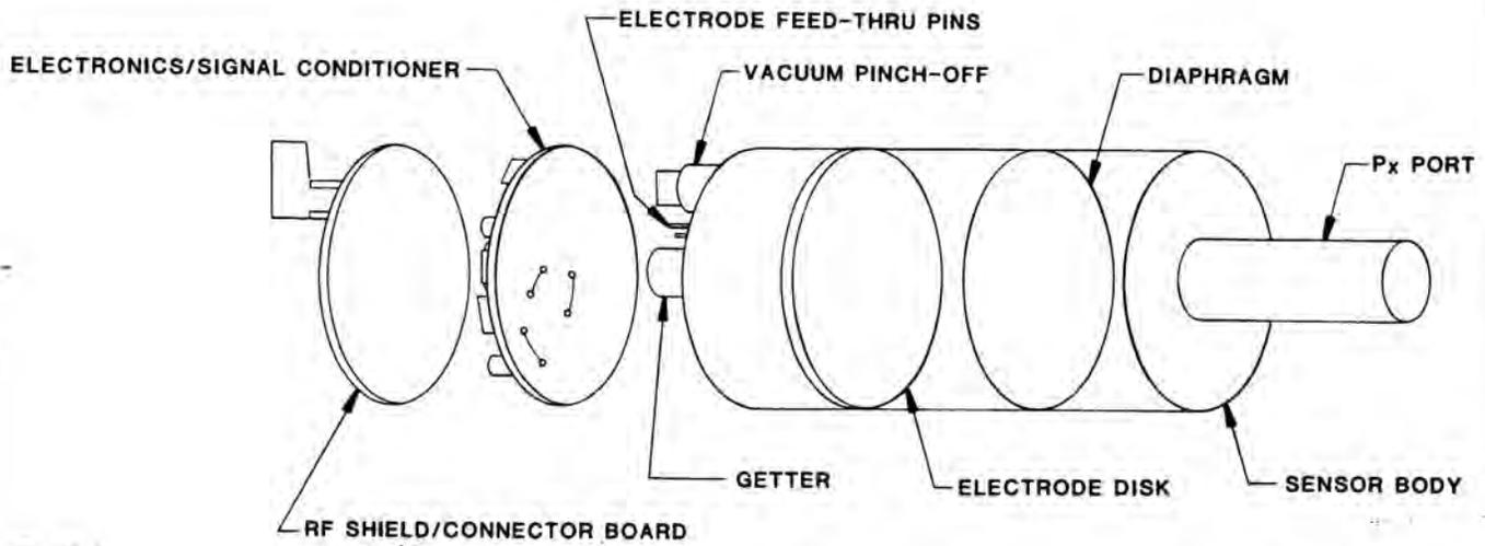
Figure 5: Cross Sectional View of the Type 122 Transducer
