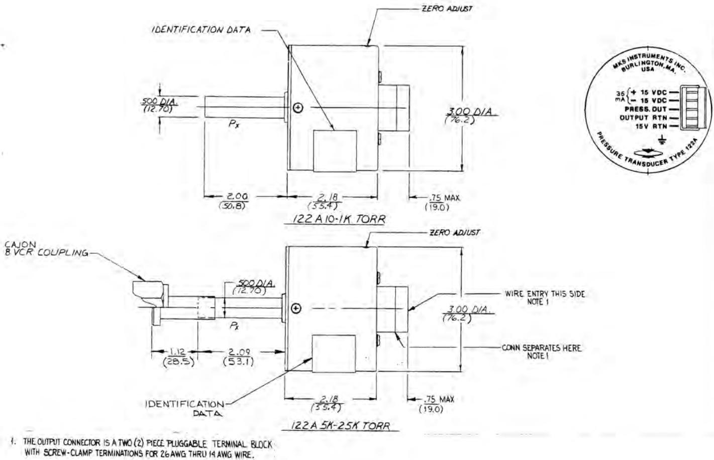
Figure 1: Dimensions of a 122 Transducer
