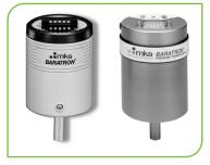
electromechanical relays that can be set to open or close at any pressure from 0.1% to 100% of the product's Full Scale measurement range. These relays can be used to control external equipment, such as isolation valves, other high vacuum gauges (such as hot-filament ionization gauges), drive motors, etc. They are available in Full Scale measurement ranges from 10 to 1000 Torr (13 to 1333 mbar).
