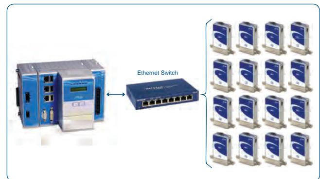
Figure 8. Ethernet-Based MFC Control Solution
