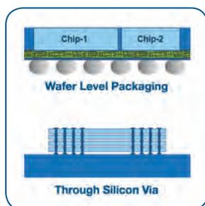
Due to the thinner nature of the wafers for advanced packages, curl and cracking occurs from routine handling. Back side grind induces stress creating wafer warp, and surface and sidewall micro-cracks are induced by traditional mechanical dicing methods. All of this impacts yield. Alternate singulation
