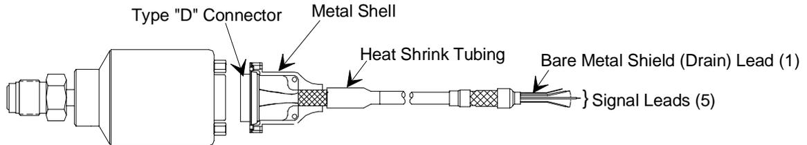
Figure 4: Components of a Cable to Connect to a Type “D” Connector
