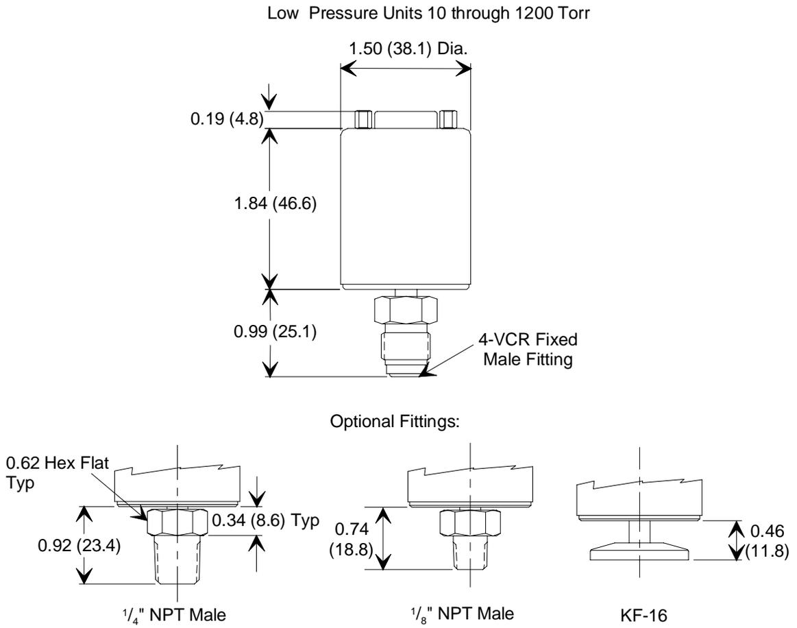
Figure 2: Dimensions of Low Pressure Single-Ended Units
