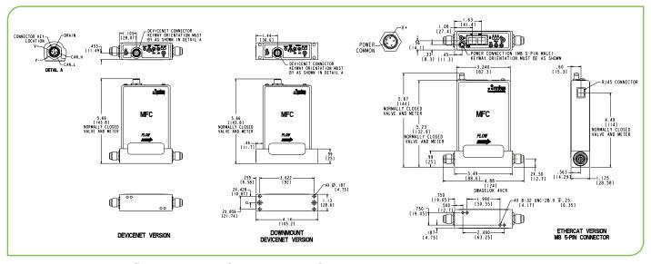
Dimensional Drawings: DeviceNet<sup>™</sup>, Downmount with VCR® fittings\* and EtherCAT® with VCR fittings\*
