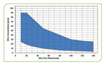
Figure 1 - Specified achievable dissolved ozone concentration in UPW for a system pressure of 2.5 bar<sub>g</sub>, a cooling water temperature and UPW temperature of 20°C. At higher UPW temperatures, lower system pressure or higher cooling water temperature, the maximum performance will decrease.
