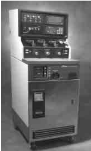
Figure 3: Self-contained portable vacuum gauge calibration system.
