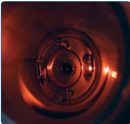
Figure 5a - MKS CIGS Ion Gauge Sensor showing sensor with filament on and degas mode on.
