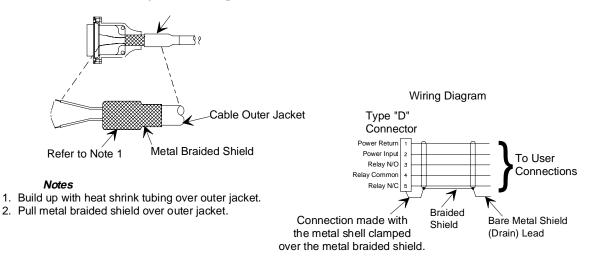
Figure 5: Expanded View of the Cable
