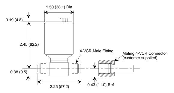
Figure 3: Dimensions of Flow-Through Units
