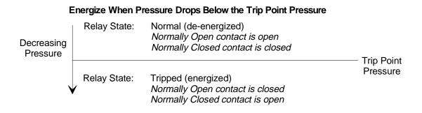
Figure 10: Trip Point Set to Energize Below the Trip Point Pressure
