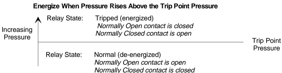
Figure 9: Trip Point Set to Energize Above the Trip Point Pressure
