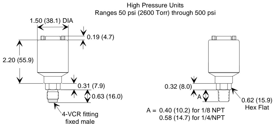
Figure 1: Dimensions of High Pressure Single-Ended Units
